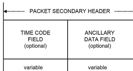
Figure 5.3 Space-packet secondary header (image courtesy of CCSDS).
