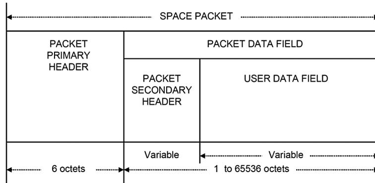
Figure 5.1 Space packet structural components (image courtesy of CCSDS).
