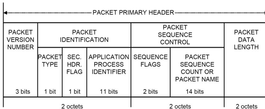
Figure 5.2 Space packet primary header (image courtesy of CCSDS).
