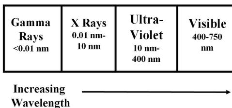
**Figure 4.1** The short-wavelength region of the electromagnetic spectrum.
