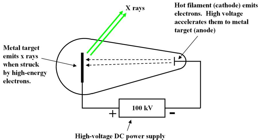
**Figure 4.3** Crookes tube schematic.
