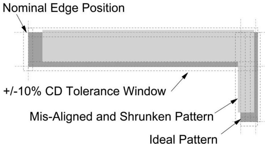
Figure 1.4 Edge placement tolerance.
