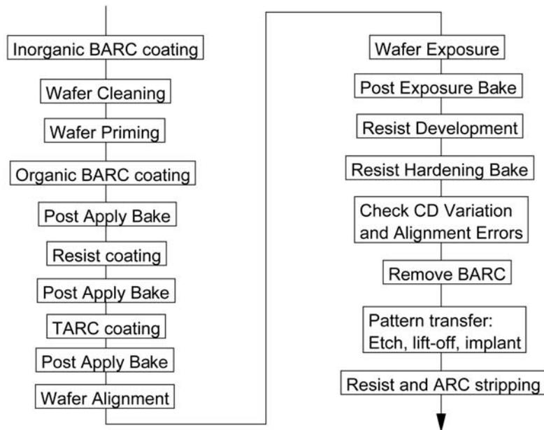
**Figure 1.3** Block diagram of lithography processing steps.
