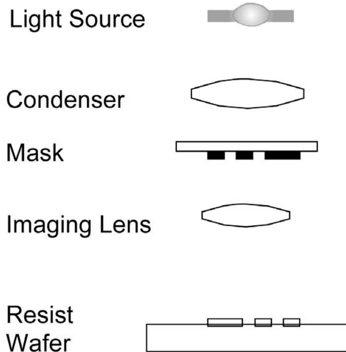
**Figure 1.1** Optical lithography replicates the mask pattern through an imaging lens.
