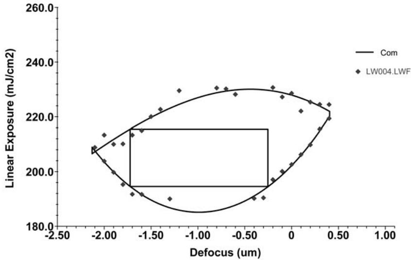
Figure 1.5 A typical E-D window in an E-D tree.
