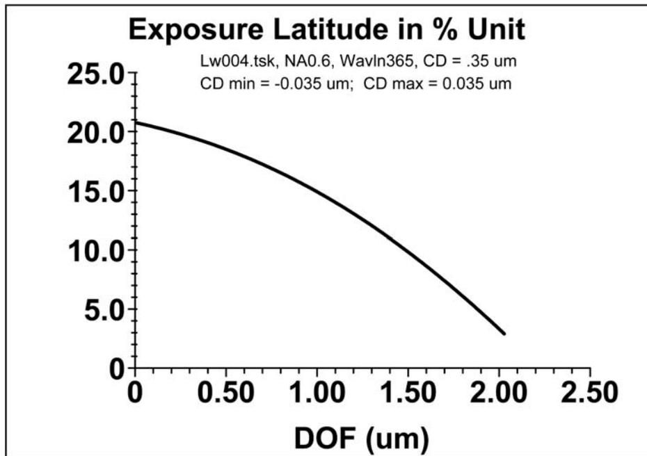
Figure 1.6 Exposure latitude versus DOF tradeoff curve.
