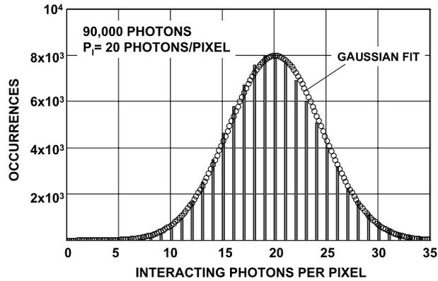
**Figure 3.6** Interacting-photon-per-pixel histogram assuming 20 photons/pixel average.
