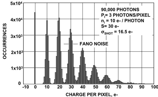
**Figure 3.9** Charge-generated-per-pixel histogram with Fano noise present ( $n_i = 10 e^-/\text{photon}$ ,  $P_1 = 3 \text{ photons/pixel}$ ).
