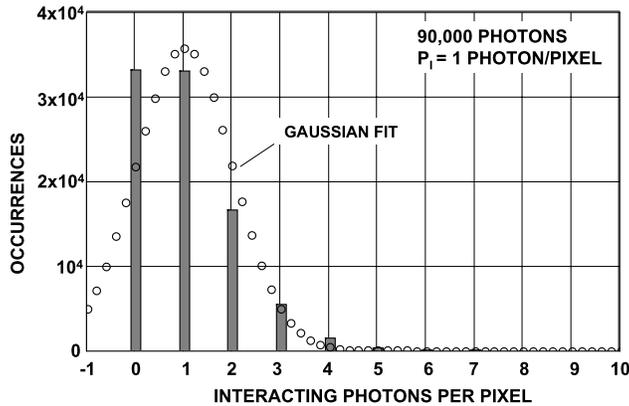
**Figure 3.3** Interacting-photons-per-pixel histogram for Fig. 3.1 assuming 1 photon/pixel average.
