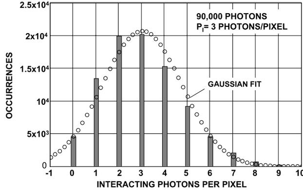
Figure 3.5 Interacting-photons-per-pixel histogram assuming 3 photons/pixel average.
