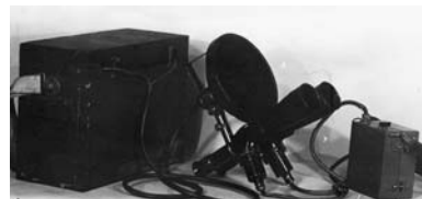
A target-designation device, an addition to the gunsight "Iskra."
