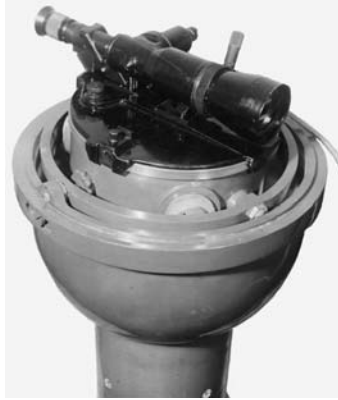
Infrared direction finder “Omega” mounted on a gyrocompass repeater.
