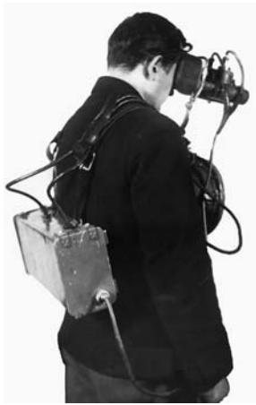
An experimental sample of the night-vision reconnaissance apparatus, fabricated at the All-Union Electrotechnical Institute in 1940, using the C-1 image converter and IR illuminator.
