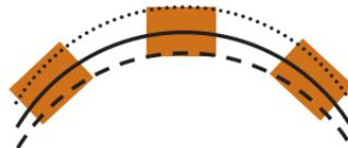
Each colored lens blank starts at same size. Initial removal is greatest, final removal least, and wedge is constantly changing on outer parts of block at constant radius.
