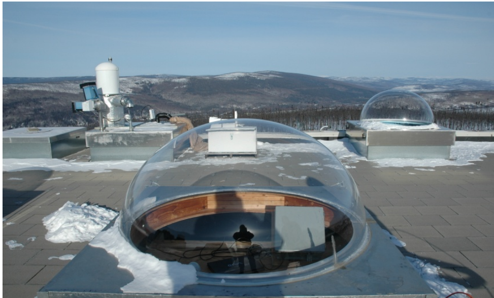
Fig. 4. Prototype optical aurora detector (gray box at lower right) deployed to view the northern horizon from a rooftop observation dome at PFRR near Fairbanks, Alaska for testing during March 2007. [J. Shaw photo].
