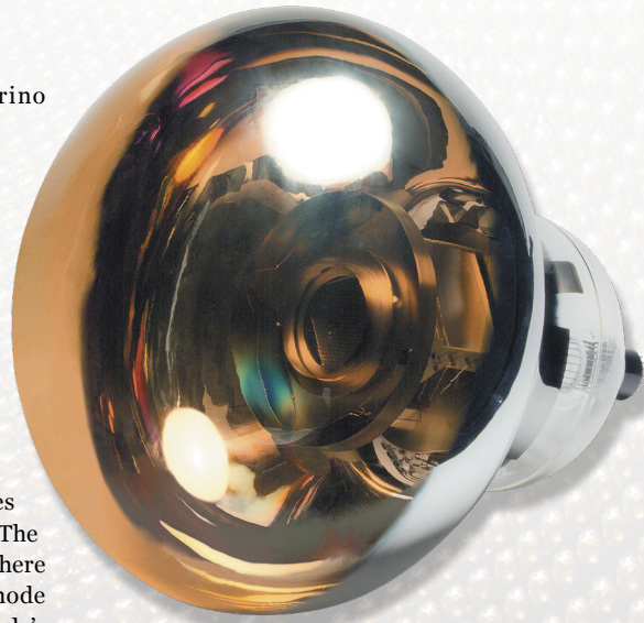
A 20-inch-diameter photomultiplier tube (PMT) for water-Cherenkov observatories such as Super-Kamiokande.
