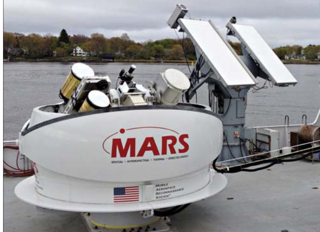
The Kineto Tracking Mounts on the MARS system can telescopically track and image aircraft, rockets, spacecraft, and other objects.
