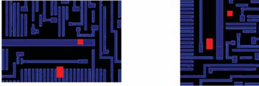
Figure 2. With space defining absorber (a darkfield mask) the layout pattern can be rotated and repositioned so that both defects fall into "harmless" areas, as shown in the right hand image.
