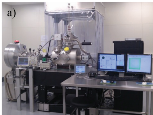
Figure 7. Photograph of the EUV laboratory exposure tool (EUV-LET) in the cleanroom environment (a). Scheme of the experimental setup with all relevant components (b).
