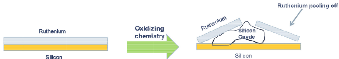
Figure 3. Silicon dioxide formation with resulting volume increase and Ruthenium peeling-off.
