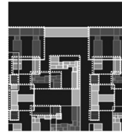
Figure 9. Example of CP extraction (Dotted squares are CPs. They are overlapping.).
