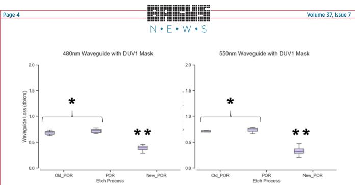
Figure 4. Waveguide propagation loss for (left) 480nm wide waveguides fabricated with the DUVI mask across the three different etch processes and (right) 550nm wide waveguides. In both charts, using a 95% confidence Tukey test, there was no statistically significant difference between the "Old POR" and the "POR" but the "New POR" did yield waveguides with significantly lower losses.
