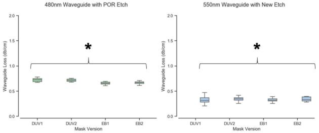
Figure 3. Waveguide propagation loss for (left) 480nm wide waveguides fabricated with the current process of record etch across the four different mask versions and (right) 550nm wide waveguides fabricated with the "new" etch process. In both charts, there was no statistically significant difference between the four groups using a Tukey honest significance test (HSD) to a 95% confidence interval.
