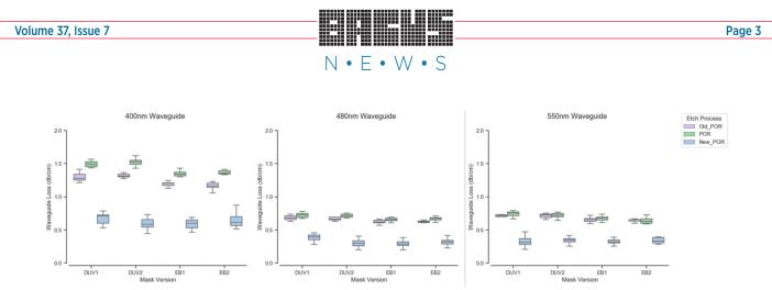
Figure 2. Waveguide propagation losses across the four mask versions and three etch processes for (I-r) 400nm wide waveguides, 480nm wide waveguides, and 550nm wide waveguides.
