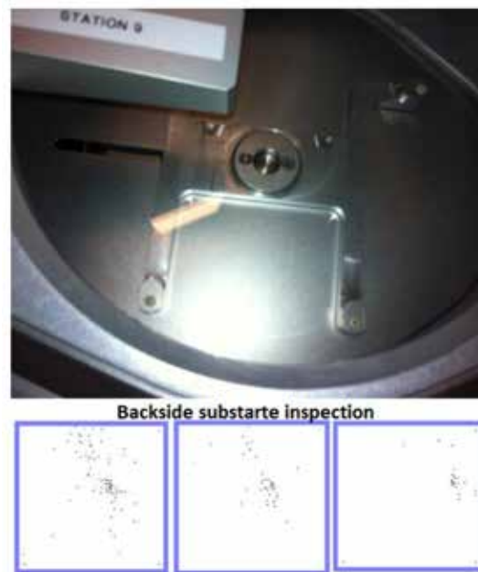
Figure 6. Aligner and several backside defect maps showing the signature of the aligner failure.
