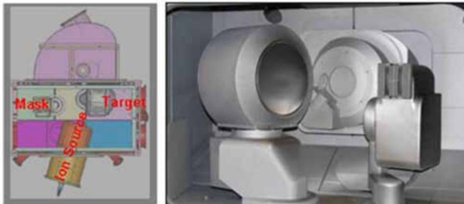
Figure 1. a) Schematic of Deposition Chamber Showing Position of Mask, Target, and Ion Source; b) Process Module at SEMATECH Showing Different Components.
