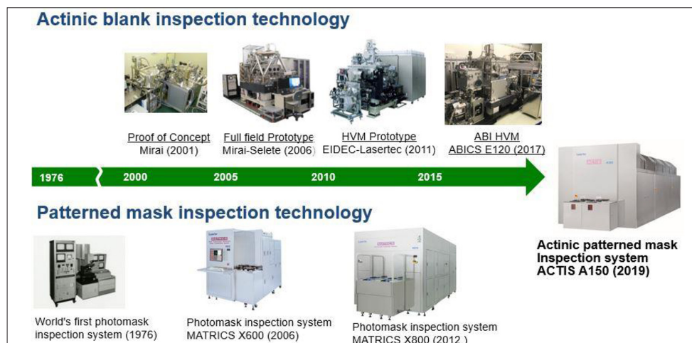
Figure 1. History of actinic blank and patterned mask defect tools leading to the APMI system.
