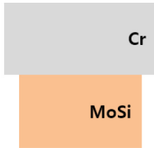
Figure 2. Structure of Mask before Cr strip.
