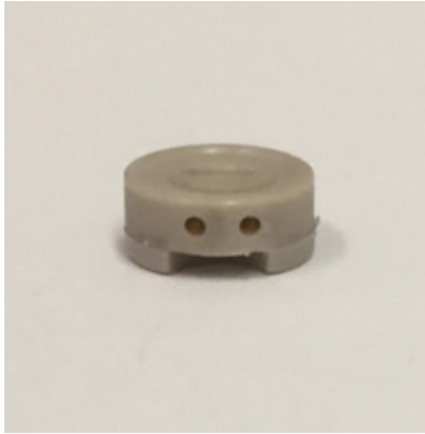
Figure 6. Current flow cell. Excess mass has been removed to push the resonant frequency of the piezo-flow cell system as high as possible.
