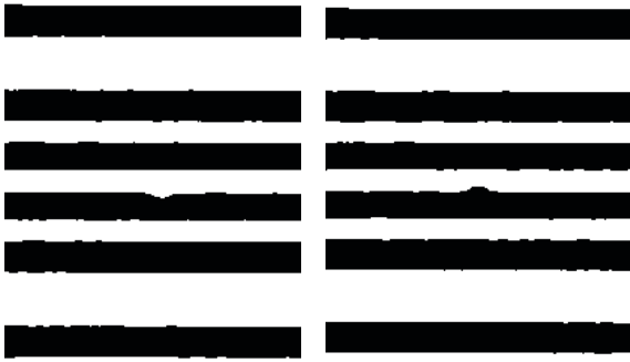
Figure 11. SEM contours of mask patterns for the maximum clear defect (left) and opaque defect (right).
