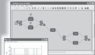
RZ-QPSK transmitter and self-homodyne receiver with QPSK signal phase plot in the time-domain
