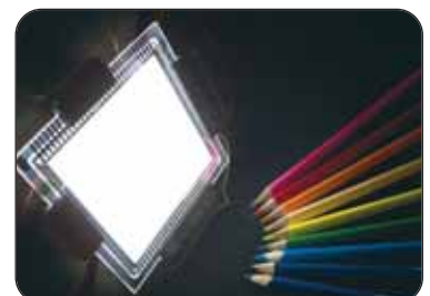
A research demonstrator of a white OLED lighting panel (source NOVALED / OLLA project).
