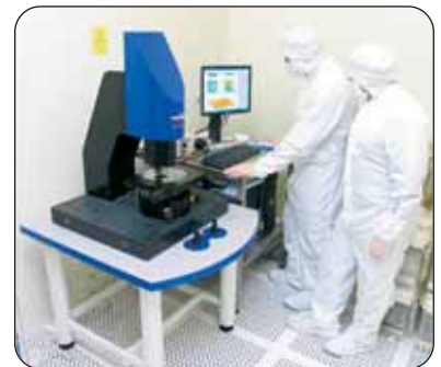
CCI 6000 ULN : the most accurate optical 3D surface profiler.
