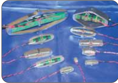
Amplified piezo actuators for large, fast and precise positioning and vibrations.
