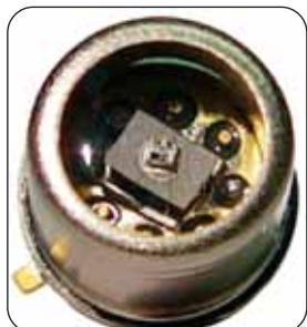
The id100-OEM, the world's smallest single photon counter.
