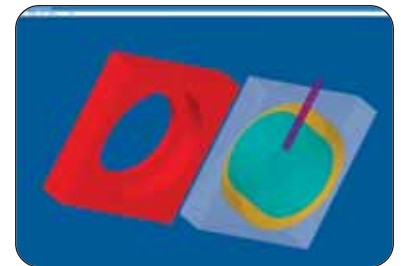
A lens mount built in ZEMAX by subtracting several cylindrical volumes from a rectangular volume.
