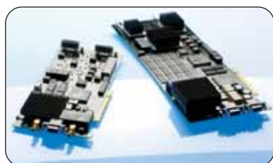
A complete picosecond fluorescence imaging system on a single PCI board.
