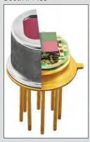
Miniaturized pyroelectric detectors – 4 channels in TO39 housing for gas analysis.
