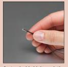
Customizable high resolution micro camera (Ø,2mm) with integrated illumination.
