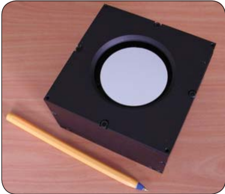
Low-cost piezoelectric deformable mirror with 109 actuators.
