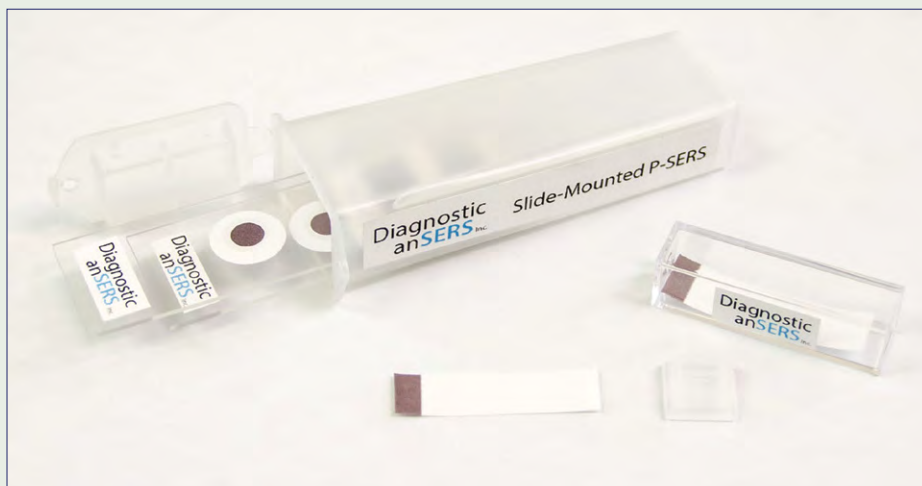
Diagnostic anSERS is developing affordable ink-jet printed SERS substrates for Raman spectroscopy.
