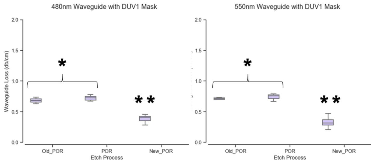
Figure 4. Waveguide propagation loss for (left) 480nm wide waveguides fabricated with the DUV1 mask across the three different etch processes and (right) 550nm wide waveguides. In both charts, using a 95% confidence Tukey test, there was no statistically significant difference between the "Old POR" and the "POR" but the "New POR" did yield waveguides with significantly lower losses.
