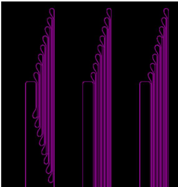
Figure 1. "Racetrack" waveguide designs.
