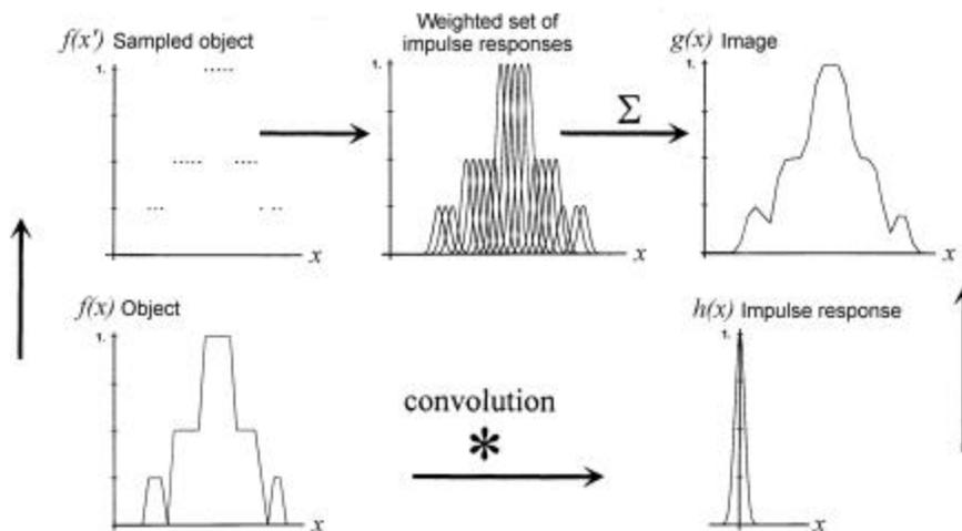
**Figure 1.2** Image formation can be modeled as a convolutional process. The clockwise loop is a weighted superposition of impulse responses and the counterclockwise loop is a convolution with the impulse response.
