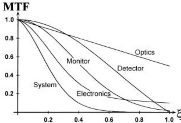
**Figure 1.7** The aggregate transfer function of several subsystems is a multiplication of their transfer functions.
