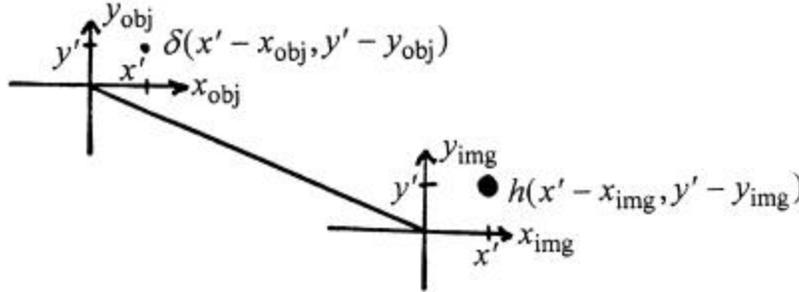
**Figure 1.1** A delta function in the object is mapped to a blur function, the impulse response, in the image plane.
