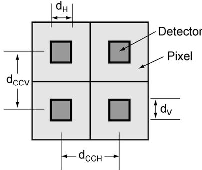
Figure 1-8. Fill Factor definition. The photosensitive area ( $A_D$ ) is  $d_H d_V$  and the pixel area ( $A_{PIXEL}$ ) is  $d_{CCH} d_{CCV}$ .
