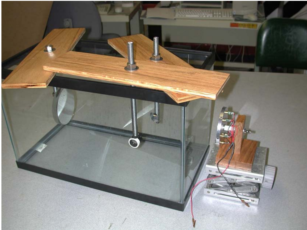
Figure 3. Top: Light path of a Newtonian reflecting telescope, as shown using the Ray Tracing demonstration system. Note that this is not a time exposure; the naked-eye image looks just like (actually better!) than this. Bottom: The setup used to produce the upper image. Note the primary and secondary mirrors, the 'eyepiece', and the laser diode array to the right.
