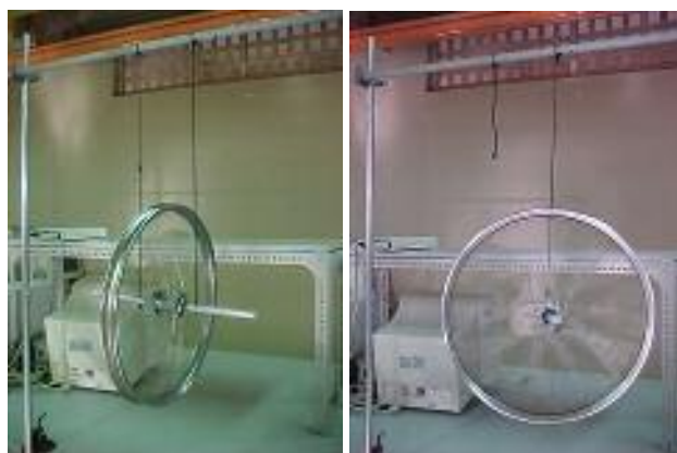
Fig. 2. An active learning module on angular momentum: what happens to the rotating wheel if one of the strings is cut?
