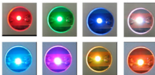
Figure 2: Coloured lights generated by the mixer (red, green, blue, white, cyan, magenta, yellow and orange).
