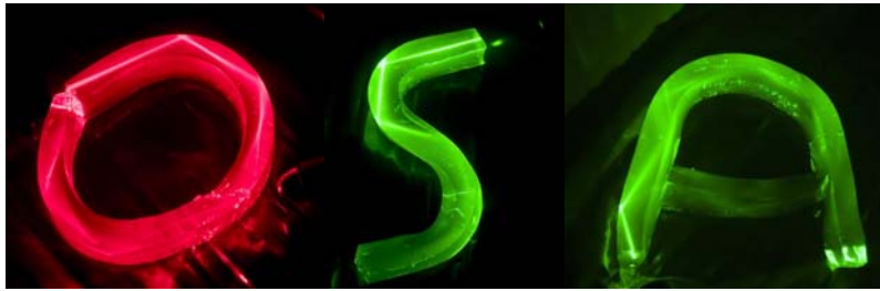
Figure 1: Total internal reflection occurring in gelatine waveguides
