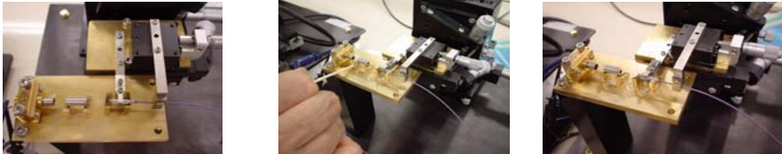
Fig. 10. Fixing the isolator, the second lens and the two wedge plates.
