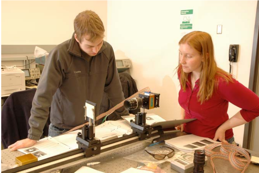
Figure 3 : Two students from the class of 2006-07 (Michael Harris and Katelyn Kern) are shown experimenting with their completed camera. The camera is the gold colored box behind the Nikon lens that is directed at a resolution target mounted on the optical rail. The students are rarely seen as serious- looking as they appear in this photograph.
