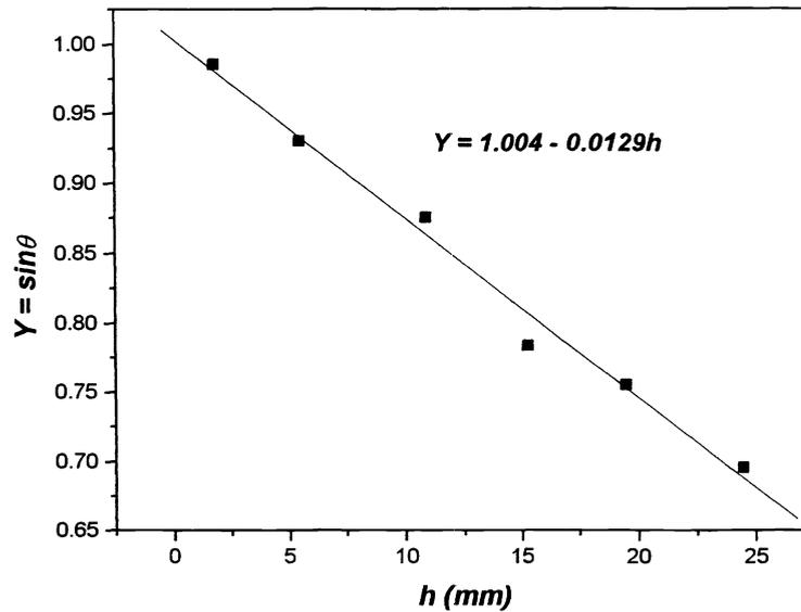
Graph 1. The sine of the incident angle as a function of the height  $h$  (see figure 7). Also, we can see the numerical fit.
