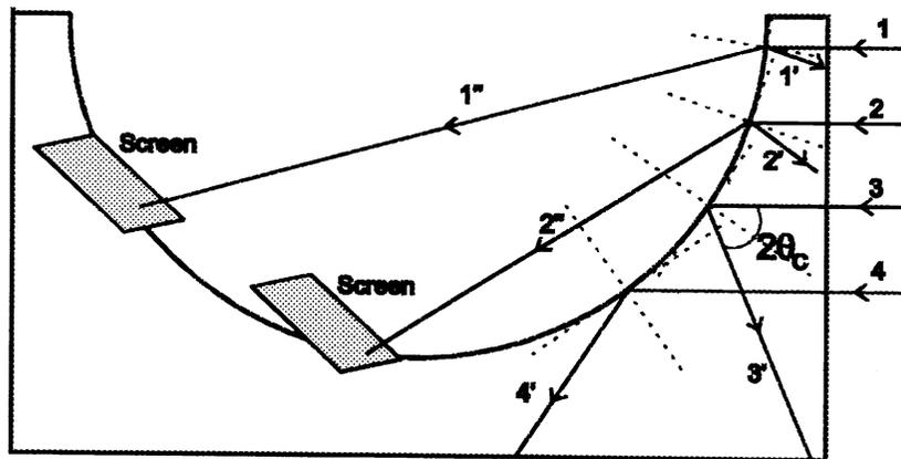
Figure 4. Transmitted beam from the material to the air followed by the screen.
