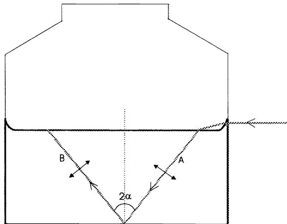
Figure 9. Reflection and refraction of light, produced by the meniscus of the liquid very close to the walls container.
