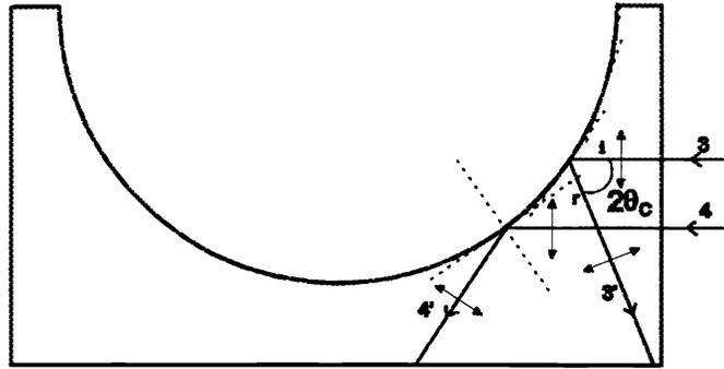
Figure 6. Light polarization by scattering when it is seen perpendicularly to the direction of the incident beam.
