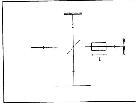
Figure 1. In one of the interferometer arms a cell is placed in order to extract the air. By this procedure, the air refractive index is measured.
