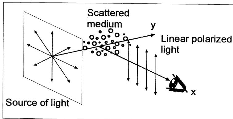
Figure 5. Linear polarization by scattering at  $90^\circ$ .
