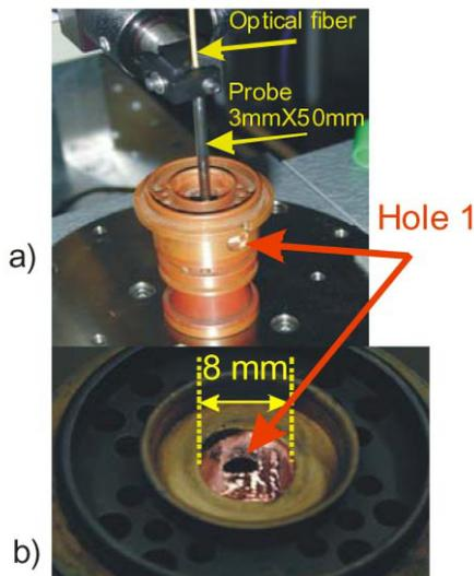
Figure 3. (a) The internal surface of the plasma torch electrode has a cylindrical shape, 8mm in diameter and 4cm long. A portion of the internal surface is visible in (b).
