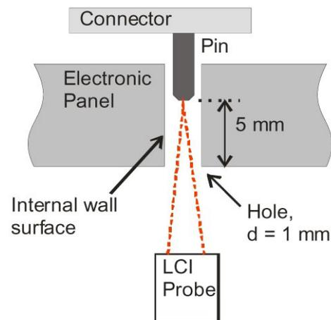
**Figure 1.** This scheme shows measurement of the insertion depth of a pin in an electronic panel. LCI: low-coherence interferometry.
