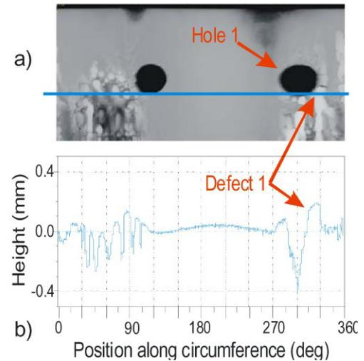
Figure 4. (a) Shown is an unfolded 3D image of the internal surface of the electrode. Depth is encoded as black (deeper) to bright values. The two holes visible in the image are aligned 180 from each other. (b) Height variations of the surface along one full circle are indicated.
