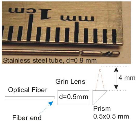
Figure 2. The optical probe is attached at the end of an optical fiber.
