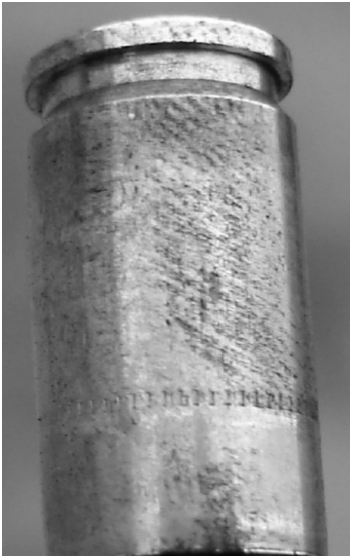
Figure 2. Ridge development visualized post-firing for fingerprint deposited on brass 9mm pistol cartridge prior to loading. The cartridge case was washed before the electric potential and conducting powder were applied.
