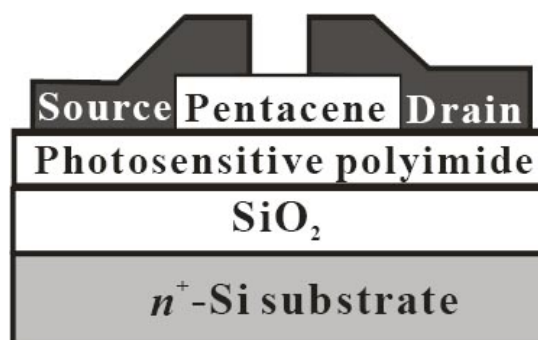
Figure 1. Cross-section of an OTFT in which the silicon substrate also acts as gate electrode. A photosensitive polyimide modification layer is inserted between the gate dielectric and pentacene films. n^+ -Si: Highly doped negative-type silicon. \text{SiO}_2 : Silicon dioxide.
