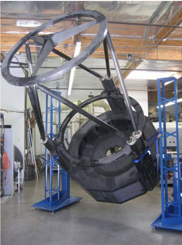
Figure 2. The OTA for the Naval Research Laboratory 1.4m telescope under construction in the shop at CMA.
