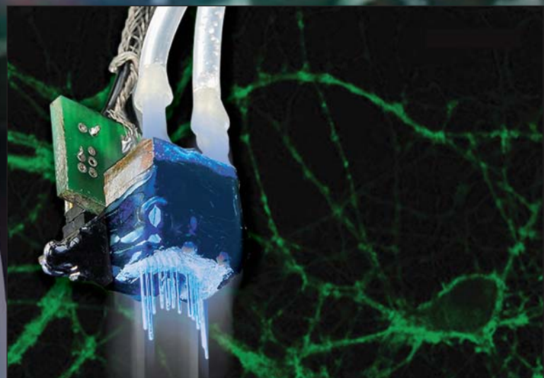
An optical fiber array for targeting neurons in a distributed pattern throughout the brain.
