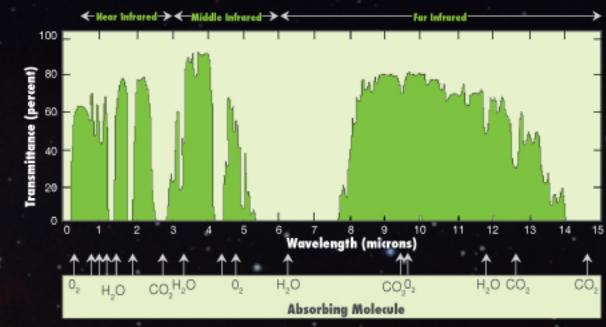
The bands of IR wavelengths that the atmosphere transmits are called the atmospheric NS: These windows vary greatly with local conditions such as water content temperature. A large gap in the absorption spectrum of water vapor, the main greenhouse gas, is most important in the dynamics of the windows. System technologies optimize operations in
