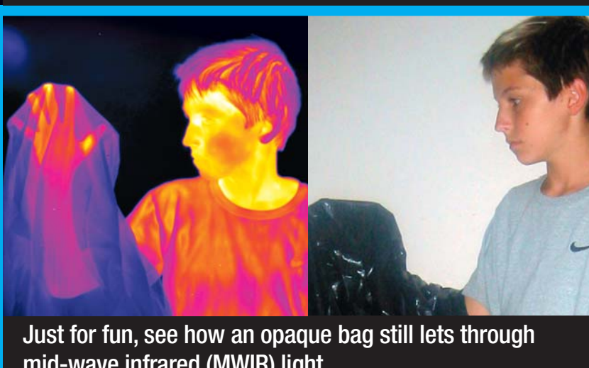
Just for fun, see how an opaque bag still lets through mid-wave infrared (MWIR) light.
