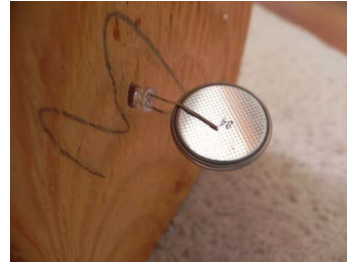
Image 4 - how the L.E.D. was lit for testing (Joshua Marino)
