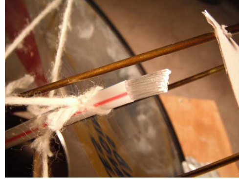
Image 10 - Fiber-Optics being filled with light from solar collector (Joshua Marino)
