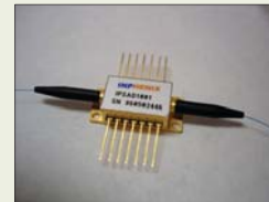
850nm/1050nm/1300nm swept light source; wavelength repetition rate 100KHz over 100nm
