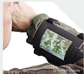
A flexible display keeps troops informed during operations with night vision, GPS, and physiological feedback.
